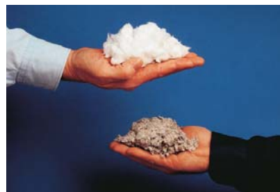
Fiber glass insulation (top) is a more fire-resistant choice than cellulose (bottom).
